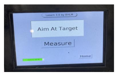
After a measurement is made the operator can choose to re-measure, accept, or foul. Re-measure will allow the operator to re-measure the current mark or a new mark without the distance being displayed on the scoreboard. Accept will send the distance displayed on the touchscreen to the scoreboard. Foul will send FOUL to the scoreboard.
