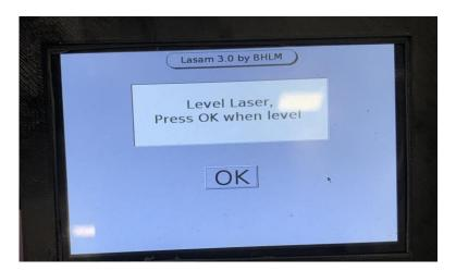
Using the vertical adjustment knob to center the bubble level on the laser module. Once level, press OK. Now follow the prompts on the screen to aim at the center of the circle or the edge of the long jump board. The measuring stick can be used for this or the included stationary point can be placed in the center of the circle. (The center of the circle should be clearly marked with a black dot, or a drilled hole. Ensure it has been properly marked by checking with a tape measure.)
