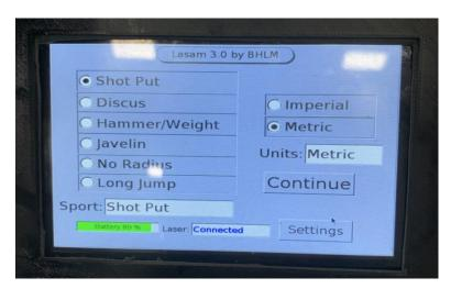
Once the home screen appears on the front touchscreen, select the appropriate event and measurement system using the touchscreen interface. Then press continue. Next, you will be prompted to level the laser.
